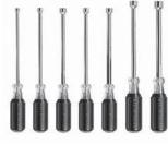
Rare Earth magnetic tip. (Only with P/N 12-01594). Full hollow shafts facilitate work on long bolt applica-tions. Cushion Grip handles allow for greater torque and comfort. Handle domes are color coded for easy identification. Internal flanges provide solid, twist-resistant shaft anchor. Chrome plated shaft helps prevent corrosion. Set contains Cat. No. 646-3/16M, 646-1/4M, 646-5/16M, 646-11/32M, 646-3/8M, 646-7/16M, 646-1/2M.
