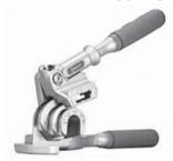
The 470-FH Triple Head 180° Tube Bender bends 4 diameters of tubing with just one tool! It handles soft copper, aluminum and thin-walled steel ald fill walled steep in 3/16", 1/4", 5/16" & 3/8" diameters. Like the heavy duty 464-FH, it features the patented ROTO-LOK<sup>TM</sup> twostage handle that allows east fabrication of bends up to 180°. It also features optimized bending grooves that allow the user to bend the tubing in the small-
