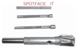
The Spotface it tool makes a flat spot for screws. This tool is specifically modified to provide rail cap clearance for use on seat rails. Cutter comes with 1/8, 5/32, 3/16 pilots. P/N 05-04429 ...... with 1/8, 5/32, 3/16 pilots.
