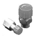
Knurled for ease of application, Series CD caps seal flared JIC fittings exceptionally well against dirt and moisture, as well as for masking during dipping, painting and plating.
