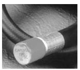
Series SC sleeve caps are designed to fit outside diameters of tubing sizes listed with a snug friction grip. Available in 57 different O.D.'s and lengths. Ideal for capping and protecting both threaded and nonthreaded tubing or rod ends. The also make excellent masks, for painting, plating or grit-blasting operations.
