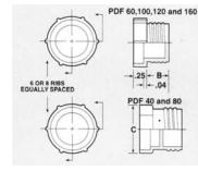
Series PDF plugs are designed for easy mechanical or hand installation on flat-faced O-ring fittings.
