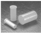
Series RCL caps are ideal for protecting threaded or smooth cylindrical surfaces. Originally designed for use on hydraulic double threaded bulkhead fittings, they are especially suitable where greater longitudinal protection is required.
