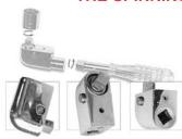
This tool is a combination tool providing a ratchet wrench for power and a spinning action for speed. All types of accessories can be used with this wrench, such as extensions on either end, or flexible drives. The drive handle can be removed to make a very compact tool for restricted areas. The ratchet pawl is made from annealed steel to allow it to fail before the ratchet
