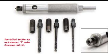
Our new Blind Rivet Removal Tool is designed to remove those stubborn Pop, Avdel, Cherry-Qt, and other blind rivets. The serrated end cups over any button head, round head, or universal head rivet and locks in place to keep it from spinning as it's being drilled out. It will also remove solid rivets. Includes adapters to remove 3/32", 1/8", 5/32", and 3/16" rivets. Not for use with steel-stemmed blind rivets.
