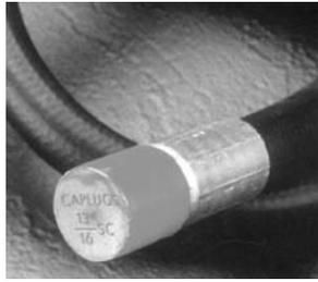
Series SC sleeve caps are designed to fit outside diameters of tubing sizes listed with a snug friction grip. Available in 57 different O.D.'s and lengths. Ideal for capping and protecting both threaded and non-threaded tubing or rod ends. They also make excellent masks, for painting, plating or grit-blasting operations.
