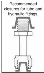
Tapered Capplugs can be used as either caps or plugs. Because they are tapered in design and made from highly pliable (or flexible) Polyethylene, they can be applied to fit snugly and are readily removable, whether used for capping or plugging. Especially recommended for use on MIL Std. and SAE-type tube and hydraulic fittings and for threaded external and internal NPT fittings.
