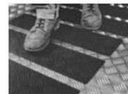
A durable, mineral coated, non-slip fabric for wing walks. Waterproof, weatherproof and unaffected by vibrations, heat, cold, gasoline or oil. Assures safe footing. Pressure-sensitive backing should have additional coating of Pliobond to assure adhesion for aircraft applications. Sold by lineal foot.
