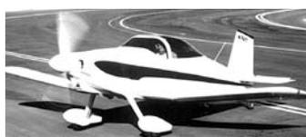
The S-18 folding wing aircraft is available as a plans or kit built aircraft. It is an all metal 2-place side-by-side aerobatic plane. The basic structure is the same as the proven T-18 Thorp with a wider and longer fuselage. Revised airfoil on the
