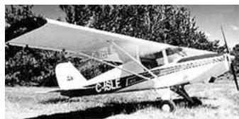
The BushCaddy was developed as a rugged Canadian bush plane that performs equally well on wheels, skis or floats. The 44 inch wide cabin, doors that swing upwards under the wings and side by side adjustable seats afford the pilot easy access and a comfortable ride.
