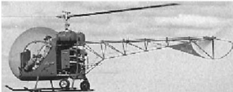
Designed for the ruggedness and reliability crucial for flying in remote areas, the Safari is powered by a Lycoming 160 Hp aircraft engine, maintaining
