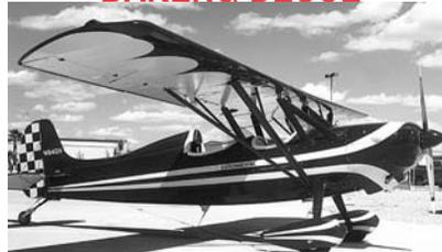
The Bakeng Deuce is a two place parasol that is great for plain every day or weekend flying. It is of a basic aircraft design utilizing a steel tube fuselage. The structure is faired with plywood and aluminum formers which support spruce stingers. Wings are of basic wooden construction with solid spruce spars. The Deuce is a very easy aircraft to build with an excellent set of plans. It has a max. speed of 140 mph, cruises at 110-120 mph with a stall speed of 35-40 mph.
