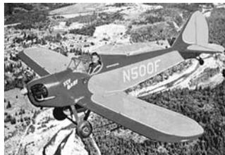
This plane is a structurally simple and easy-to-fly airplane designed to the requirements of the Experimental aircraft Association for home construction and storage in a space 7' x 8' x 20', which is equivalent to the standard home garage. Great emphasis has been placed upon safe flight characteristics and good low speed performance for takeoff and landing at some sacrifice of high speed. The
