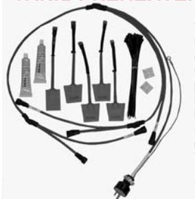
Preheat your Jabiru engine in cold weather for faster and safer starts. This system directly heats the cylinder heads and oil sump. The kit includes all heating elements, wiring harness with 120 volt power plug, instructions, and complete installation materials. Cylinders are heated with elements that bond to the rocker covers. Available for four and six cylinder engines.
