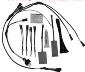
Rotax 912 Engines - Preheat your Rotax 912 engine in cold weather for faster and safer starts. This system directly heats the cylinder heads, crankcase, and oil reservoir. The kit includes all heating elements, wiring harness with 120 volt power plug, instructions, and complete installation materials. Cylinders are heated with the exclusive Tanis heated bolts that take the place of the Allen head cap screws that secure the rocker covers.
