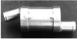
Universal air-oil separator ideal for virtually any experimental aircraft. They are machined from aluminum stock and welded by a certified welder. Oil separation is provided by baffles attached on the inside. This is a one pipe system with no extra drain lines or hoses required.
