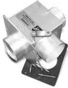
This cabin box is a modification of our popular standard heat box. Re-engineered as a one-piece unit with two tube-end outlets, rather than one tube-end outlet and one flush outlet; it is smooth, efficient and very light. Originally designed for use on the popular RV series of aircraft, it is applicable to most homebuilts. They are constructed of aircraft grade aluminum and weigh only 5.5 oz. The new design
