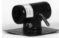
Custom built aluminum box mounts to firewall. Lever on butterfly may be attached to push-pull control for close adjustment of cabin air flow. Two 2" intake ports, one 2" outlet. Wt. 1 lb. 7-1/2" long. Fine quality construction.
