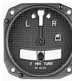
Built-in voltage regulator allows it to be used in either 14V or 28V systems. Small, compact unit and weighs only 1.2 lbs. Incorporates a small "power out" warning window which is black when normal current is being supplied but turns red in the case of electrical power failure. This turn and bank is now being used in many production aircraft. New installation requires electrical connector and cable clamp. New manufacture by Electrical Gyro Corp. Size: 3-3/8" x 3-3/8" x 3-3/4" long.
