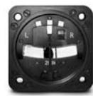
The unit is an electrically-driven gyroscope. The inclinometer, by movement of a ball in relation to the lubber lines, indicates the slip angle of the aircraft while in a turn. A power flag drops into view whenever the voltage drops below a level which is required for proper operation of the gyro. It incorporates a built-in voltage regulator so it can be used with either 14VDC or 28VDC power supply system. It has a DC-AC-DC converter. Power Supply: 10-30VDC, Electrical Consumption:
