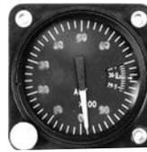
The mini altimeter is a remarkable instrument. Through the use of an accurate single pointer design, the 0-5,000 and 0-10,000 altimeters are able to squeeze precision and reliability into a 2-1/4" instrument which is less than 2" deep. All altimeters are designed with Kollsman windows, glass faces, precision jewelled movements and a rugged combination metal and plastic case. Static porting is standard.
