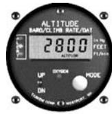
The Series 2000 Digital Altimeter is a precision instrument providing altitude readings from -100 to +30700 feet in 10' steps. A standard 3-1/8" instrument powered from 11-35V DC & uses a highly visible backlit liquid crystal display. Displayed data includes Altitude, Baro Ref & Vertical Speed. A programmable altitude alert function combines both audio and visual (LED) outputs. An oxygen alert cautions when over 12500 feet. All data is output in computer compatible RS-232 format.
