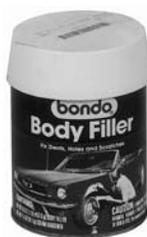
Automotive body filler, used extensively in composite construction to hold jig blocks in place, and for other temporary fastening jobs. Hardens quickly and can be chipped off without damaging the fiberglass. The color of the mixture is used to judge how fast it will set. As more hardener is added, the brighter in color the mixture becomes and the faster it hardens.
