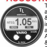
TL-3624 is suitable for most aircraft whether they be airplanes or whether they be gliders. • Measure climb & descent rate with high level of accuracy using the integrated or averaging memory with selectable averaging time • Set value limits at 2 levels (Warning & Alarm) for climb and descent rate • Use acoustic climb & descent rate signals using an external loudspeaker. Size: 2-1/4"
