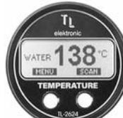
• Use the thermometer to measure up to 4 temperatures and oil pressure • Use the automatic choke function using the modeler's servo regulated by thermometer according to any of the measured temperatures e.g. CHT • Set value limits at 2 levels (Warning and Alarm) for all measured values. In case these values are exceeded the instrument will warn you at time of any possible engine damage
