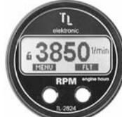
• Measure rotations & engine hours with the option to trigger the counting from a certain engine rotation rate (by your choice) so that you can divide taxing from flight time • Set value limits at 2 levels (Warning & Alarm) for all measured values. In case these values are exceeded the instrument will warn you in time of any possible engine damage • Several separate users with pilot/student option
