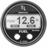
• Measure immediate fuel flow of your engine in liters/hour or liters/100 km and average fuel consumption • Set limit values at 2 levels (Warning & Alarm), for all measured values. In case these values are exceeded, the instrument will warn you prior possible failure or damage of the engine • Display at any time the fuel levels in the left, right or both fuel tanks. Size: 2-1/4"
