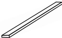
A 6-ft. long kiln-dried spruce board, 7/8" to 1" thick and 3" to 4" wide, used for checking the straightness of flying surfaces during composite construction.
