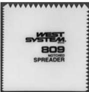
This plastic spreader is excellent for spreading epoxy at a steady rate to provide an even surface. Measures 4" x 4" and is notched on three sides in increments of 1/8", 3/16", 1/4".
