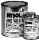
This new and improved Hysol glue replaces the old EA-9410-2 glue. EA-9430 has the same characteristics as the EA-9410, but has a 50 minute pot life instead of the 30 minute pot life of the EA-9410 at 77°F. Used extensively in the Strojnik S2A sailplane and many other homebuilts.
