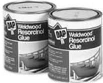
Resorcinol glue is a waterproof two-part system that meets or exceeds the requirements of MIL-A-46051 (Type I, Grade A), (Type II, Grade C), & MIL-A-22397 (Grade A). It resists outdoor exposure, cold or boiling water, heat, molds, and solvents. Pot life: 3-4 hrs. Mix Ratio: 4 to 1 by weight. Excellent for use on wood structures. 1 pint. P/N 0227...../ea
