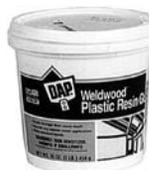
Weldwood Plastic Resin glue is a powdered, pre-catalyzed water-activated glue designed to provide strong, durable bonds for wood and wood products. Forms a bond stronger than the wood itself. Meets Fed. Spec A-A-3052.. Pot life: 4-5 hrs @ 70°, 2.5hrs @ 80°. Mix Ratio: 5 to 2 by volume. Resistant to fungi, bacteria, oil, gasoline & solvents.
