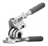
The 470-FH Triple Head 180° Tube Bender bends 4 diameters of tubing with just one tool! It handles soft copper, aluminum and thin-walled steel tubing in 3/16", 1/4", 5/16" & 3/8" diameters. Like the heavy duty 464-FH, it features the patented ROTO-LOK™ twostage handle that allows east fabrication of bends up to 180°. It also features optimized bending grooves that allow the user to bend the tubing in the small-
