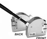
The Porto-Metal Former makes the specialty angle needed in minutes. Can be used on the work bench or in a vise to make inside angles, outside angles, straight bends even circles, to a radius as small as 3". Jaws are made of hardened alloy steel. Works 18 gauge soft steel, 20 gauge stainless, 16 gauge aluminum up to 2" in width. 45 to 1 leverage for powerful press. Special
