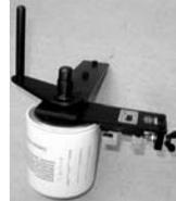
This tool was designed to eliminate much of the mess that occurs with small handheld oil filter cutting tools. Very simple to operate, it is excellent for individual aircraft owners as well as FBO's and maintenance shops where a lot of filters need to be cut. Simply clamp in a vise, screw on the filter, turn the cutter into the filter and hand crank to open the filter. The rugged construction enables this tool to operate trouble free for years. P/N 12-00122 .....
