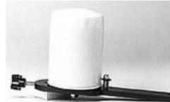
This aviation oil filter cutter will open any size oil filter canisters for your inspection. To use the tool, place the filter in a vice, attach the tool to the top of the filter, and rotate 4 to 6 turns to open the canister. The cutting wheel will stay sharp for about 50 uses, and is easily replaced when dull. The tool is made from 6061 aluminum with
