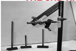
A simple yet rugged tool, The 3rd Hand was designed to hold round or square tubing in place during the welding process. Originally used for aircraft engine mount and airframe fabrication work, it has many other applications. This steel fixture is infinitely adjustable due to its full swiveling clamp. Each model comes with 3 different length arms (3.5", 5.25" & 7.5") Hose clamps are not provided.
