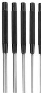
Our Drive Pin Punches have been machined to exacting tolerances for accurate driving without damaging the pin or hole. The punch ends are ground square to sit flush on the top of the pin. Made of hardened tool steel with a knurled body, General's Drive Pin Punches can either be held by hand or with our Punch and Chisel holder. This five-piece set features extra-long 3-1/2" shafts for reaching deeply recessed pins.
