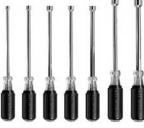
Rare Earth magnetic tip. (Only with P/N 12-01594). Full hollow shafts facilitate work on long bolt applications. Cushion Grip handles allow for greater torque and comfort. Handle domes are color coded for easy identification. Internal flanges provide solid, twist-resistant shaft anchor. Chrome plated shaft helps prevent corrosion. Set contains Cat. No. 646-3/16M, 646-1/4M, 646-5/16M, 646-11/32M, 646-3/8M, 646-7/16M, 646-1/2M.
