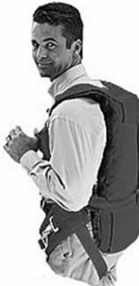
An extremely comfortable State-of-the-art lightweight emergency parachute system designed to fit into the restricted cockpits of today's aircraft. The steerable conical canopy is designed for a 240# maximum suspended weight. System size and weight 2"x15" w. x 24" long. 14 lbs.
