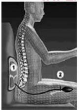
This inflatable air pillow can be installed just under the seat material and will give you the customized support just where you need it. A convenient palmsize pump and a release valve control the firmness of the lumbar support. The In-Flight Back Support is made of a heavy duty self-extinguishing neoprene rubber, specially designed to pass FAR 23.853 flame-test requirements.
