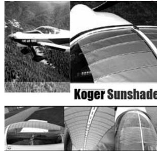
The Koger Sunshade was developed to provide protection from the sun while flying an airplane that has a large bubble plastic canopy like the RV-6, RV-7, RV-8, RV-9 and many other types of aircraft.
