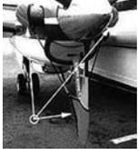
Propeller Slings & Exhaust Covers keep your propeller secure and in place, eliminating any bearing damage caused by a free-spinning propeller with no lubrication. The integral exhaust covers protect the costly turbine wheel from debris & birds. Simple, quick one man operation. Please specify aircraft make, model, serial no. when ordering.
