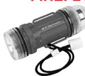
The Firefly Plus is a flashlight/emergency locator strobe which is visible for over one mile. The operating life of the strobe is 10 hours, and 2 hours for the flashlight (continuous). Firefly Plus operates on 2 AA batteries (not included) and made of durable ABS plastic. Waterproof & weighs 4 oz. Size: 2" dia. x 5-3/8"h. Excellent addition to any aircraft or home emergency kit. P/N 13-54050 .....
