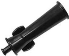
**VENTURI** - Black molded plastic venturi mounts on fuselage bottom and produces required suction to horn and outlet tubes for fluid ejection.
