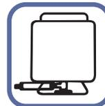
**4-Valve** Unscrew Kwik-Charge™ end fitting & reverse, then connect to refrigerant fitting as shown (flow arrow on body points upward).
