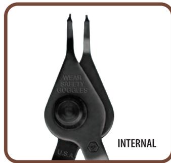
To convert pliers to internal or external position, remove thumbscrew. Pull handle halves apart and reposition screw in other hole; then finger tighten.
