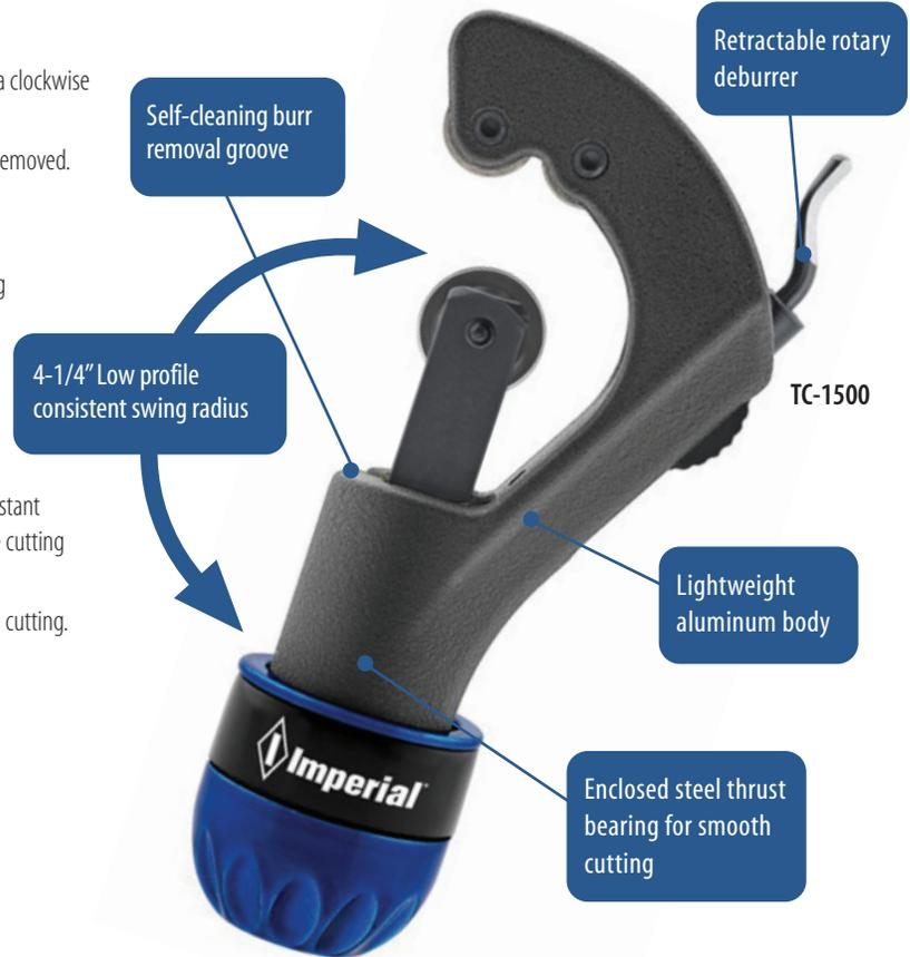
**TC-1500** For 1/8" to 1-1/8" (4 mm to 28 mm) O.D. tubing. Includes (2) S75015 general-purpose cutter wheels. Length 5". Wt. 8.0 oz.
