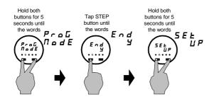
Setting Tank SIZE for the first time. Hold the STEP button in and power up to see and set size or use procedure below.
