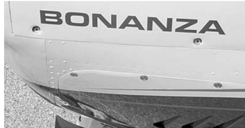
Great looking kits for converting Bonanza cowlings to the eSuperior MilSpec C-LOCK fasteners. Convert any Bonanza main engine cowling from the original Dzus fasteners to the heavy duty MilSpec 4000 series C-Locks. Convert early Bonanza gill (cheek) panels from Airloc to the MilSpec 2700 series fasteners. Convert later Bonanza gill (cheek) panels to the heavy duty MilSpec 4000 series C-Locks.
