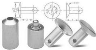
A-LOCK fasteners are common to Beechcraft airplanes and latches on many cowlings. The design consists of a simple stud, with a pin pressed into the shank. The pin is installed after inserting the stud through the panel hole and removed
