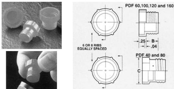
Series PDF plugs are designed for easy mechanical or hand installation on flat-faced O-ring fittings.
