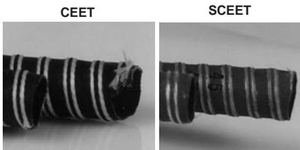
**"CEET"** - "CEET" type ducting has two plies of neoprene-impregnated fiberglass, similar to CAT except wire between plies. For use in hot or cold air applications and for conveying fumes at temperatures ranging from -65° to over 350°F. Not recommended for handling liquids or highly abrasive materials, or for negative pressure applications.
