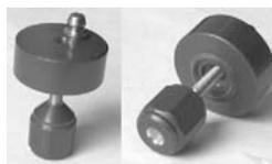
The ACS bearing regreasers restore bearings, rod ends and pulleys to "like-new" condition. O-ring in base of regreaser provides positive seal when bearing is secured by the threaded center post. Grease, entering under pressure at the grease fitting, is forced to flow through the bearing, flushing out the old grease and dirt, and recharging the bearing with fresh grease. Anodized aluminum construction. Available in five sizes.
