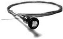
Provides a 10-lb. locking force for light and medium service applications. Black or Red anodized aluminum knob with aluminum release button. Has .062" dia. stainless steel wire core in flexible metal casing. May be shortened as req. Max. travel 3-1/2". Order by Part No.
