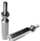
Use these stainless steel extensions for moderate length adjustments to stock length controls. Stocked with 1 male & 1 female threaded end. The extensions provide the required increase in control length when threaded approximately half way onto the control. Furnished in 2", 3", 4", 5" and 6" lengths. All extensions have 10-32 threads. To order, add -2, -3, -4, or -5 to
