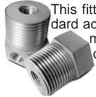
This fitting eliminates the need to put an angle fitting on standard adapter. 1/4" female pipe thread on side and bottom & 1" male pipe or 3/4" male pipe on bottom. Use with AN867-6 or 8.
