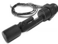
Float-action sensor in tank activates panel warning light when fuel supply is low. All-PBT unit, impervious to aviation fuel. Use AN 867-4 flange for mounting.
