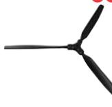
**Warp Drive's Advanced Composite Carbon Fiber propeller has a structural strength near that of metal propellers.** Because of the stiffness achieved by using carbon fibers, the prop will do very little coning (bending forward) under power. Proper fiber placement allows the prop to flex torsionally for maximum cruise efficiency. The strongly fixed position of the blades along with optimum torsional performance translates into more thrust than conventional propellers.
