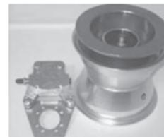
The MH6B is a 6" wheel with 5.375" width with an additional 1.24" caliper spacing. Bearing spacing is 2" and axle spacing is 2". The total weight of this wheel and brake assembly is 4.4 lbs. The bearing axle diameter is 0.625". The NEW MH6B is now produced as a CNC spun wheel with a Tenzalloy hub center and a NEW higher torque caliper. Torque Rating (@450 PSI):1540 in-lb. StaticCapacity:660 lbs.
