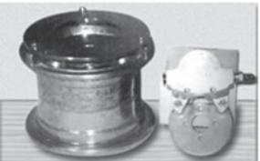
The W50CC is a 5" wheel with a 3.7" width with an additional 1.75" caliper spacing. Bearing Spacing is 3.0" and axle spacing is 2.5". The total weight of this wheel and brake assembly is 4.5 lbs. excluding the axle assembly. This wheel uses a "Lamb" type tire which is 11x400x5 and requires a tube with a 90 degree valve stem. Torque Rating (@450 PSI): 1540 in-lb.
