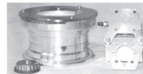
MATCO mfg produces a superior 6" wheel and brake assembly for use with aircraft requiring less than 1420 lbs per wheel. This model uses 1.25" TAPER/ROLL bearings. The W60 is a 6" wheel with 4.375" width with an additional 1.23" caliper spacing. Bearing spacing is 2.5" and axle spacing is 1.25". The total weight of this wheel and brake assembly is 7.1 lbs. The bearing axle diameter is 1.25".
