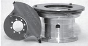
The W51LT/LXT is a 5" wheel with a 4.775" width with an additional 1.23 inch caliper spacing. Bearing spacing is 3.084" and axle spacing is 1.00". The total weight of this wheel and brake assembly is 9.2 Lbs. The bearing axle diameter is 1.25". Torque rating is 4266 in-lb for the W51LT and is 6143 in-lb for the W51LXT. W51LT is recommended for Cozy Mark IV and the W51LXT is used on the Glasair.
