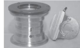
The W600XT is a 6" wheel with 6.3125" width with an additional 1.37" caliper spacing. Bearing spacing is 3.42" and axle spacing is 1.78". The total weight of this wheel and brake assembly is 11.9 lbs. The bearing axle diameter is 1.50". Torque Rating (@450 PSI): 6441 inlb. Static Capacity: 1860 lbs. Load Limit: 5580 lbs. Order axles separately.
