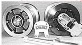
A quality built 6" wheel & brake designed for the homebuilt and ultralight flyer. Rated up to 2500 lbs. gross weight, these wheels easily accommodate 800 series tires for off-field landings and 600 series tires for low profile and an increase in speed. The brake disks made of cast iron
