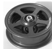
Tail wheel, fully CNC machined, static load: 330Lbs, for tyre 200x50 • Aluminum anodized Tailwheel • for 200x50 or 200x65 tube type tyre • In 2 parts easily removable, with ball bearings • Alloy: 2017 (AU4G) machined from billet on CNC • For axis 08 mm (0.32") • Weight: 9oz. P/N 06-00957 .....
