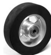
This is a replacement tail wheel for the Van's tail wheel assembly. The hub is made from 6061-t6 aircraft aluminum with a tire molded from 65 durometer SBR rubber. The design includes precision sealed bearings. 5-1/2" Diameter X 1-1/2" Thick P/N 06-01284.....
