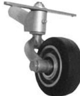
Locks in steerable mode when aircraft is moved forward. Releases to full swivel when pushed sideways or backwards, or when maneuvering on the ground using brakes. Tire is solid soft rubber, with sealed ball bearings.
