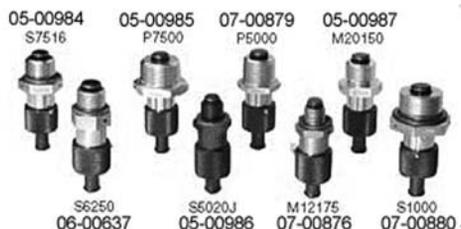
Changing hot engine oil has never been easier! With the SAF-AIR oil drain valve, no wrench is needed to remove the drain plug. A simple push and turn of the SAF-AIR valve locks it in the open position. The valve is made completely from anodized aluminum and stainless steel components. These materials are used throughout the aircraft industry due to their strength and durability. FAA & PMA APPROVED.
