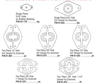
Two piece shields for use over cables or wires with large end-fittings or existing installations. Single piece for use where the cable or wire may pass through the hole. Flat shields designed for use on wooden or composite firewalls using a fire resistant sealant to prevent leaks. Both types of shield available in flat or with dimple to accommodate rubber grommets up to outside diameter.
