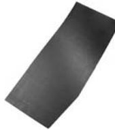
ABS thermoplastic fire-rated sheet material can be used as a base material for making of glare shields and side panel backing. Easily cut, drill, saw, and grind this ABS sheeting. The plastic sheets have an excellent ductility and formability. Meets FAR 25.853 burn requirements. Smooth flat surface on one side and a matte finish on the other side. Color: Black. Sheet size is .063" x 23.5" x 54'.
