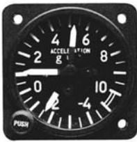
Accelerometers register to "g" forces acting on the airframe during turbulence or aerobatic maneuvers. One pointer gives a continuous reading, the other two indicate maximum positive and negative loads. Easy to reset by pushing the "push to reset" knob.
