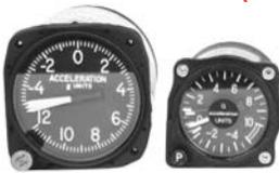
This instrument registers "G" forces acting on the airframe during turbulence or aerobatic maneuvers. One pointer gives a continuous reading, the other 2 indicate maximum positive & negative loads. A reset knob is provided. In smooth, level flight the instrument indicates +1 "G". Large "G" Meter - Range: -5G to +12G.
