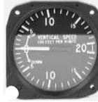
The vertical speed indicator is a precision instrument which provides an accurate indication of rate of change of altitude. This instrument is temperature compensated and is provided with a zero adjustment screw on the face of the case in the seven o'clock position. Power: Static system.
