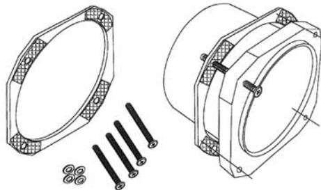
Take the frustration out of mounting instruments with the use of Superior Panel Technology's EZ Nuts. Adhesive tape securely holds nut ring in place. No realignment if instrument is later removed. Includes four
