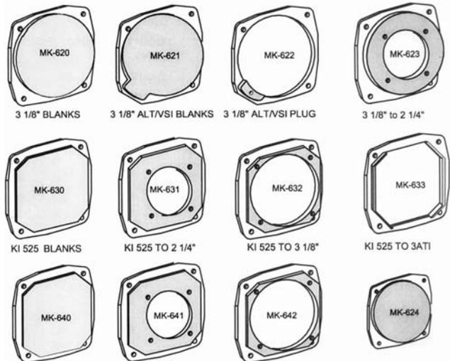
CNC Machined from aircraft grade aluminum. The adapter face is raised .075" to give the flush panel look. Easy to install and easily painted.
