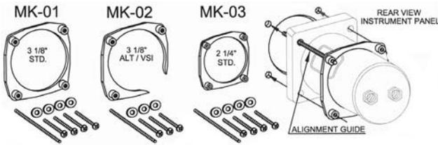
Kits come with "special" self-locking black pan head screws nylon washers, and alignment guide pin.
