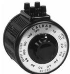
A fine quality control to supply the electrical current for hot-wire cutting of styrofoam & PVC foam. One unit can serve to build many aircraft. Input 115VAC Output variable from 0-130VAC at 5amps Caution - fuse should be inserted in the secondary to protect the control in the event of a short circuit.
