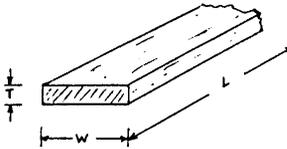
Faster delivery can be assured if guidelines regarding minimum acceptable lengths are provided. Orders are often delayed awaiting delivery of lumber to the even footage specified whereas shipment could be made if the minimum usable lengths were indicated. Example: 3/4" nominal 6" x 12' (131-1/2" min.).
